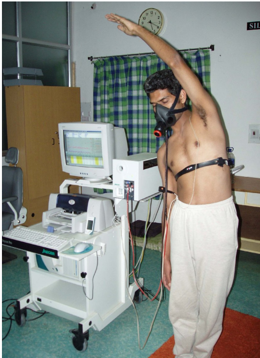
Subject in air conditioned room wearing breathing mask connected to O 2 analyzer through twin tube
