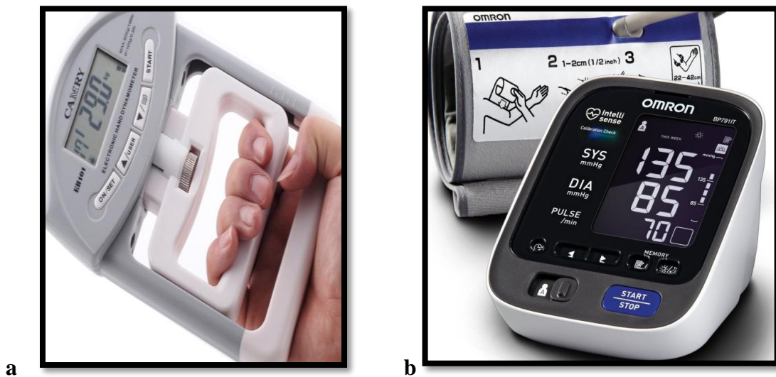
Plate 2. Images of equipment used in sympathetic reactivity tasks. a. Camry Hand grip dynamometer; b. Omron Automatic blood pressure machine.
