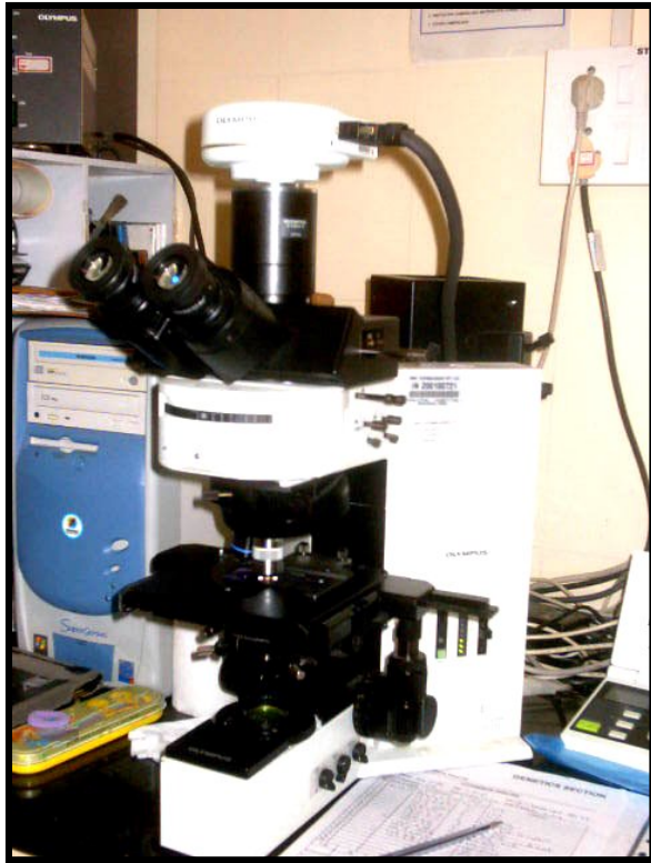
Figure 4: Trinocular Microscope with fluorescent filters used for counting cells stained with Propidium Iodide
