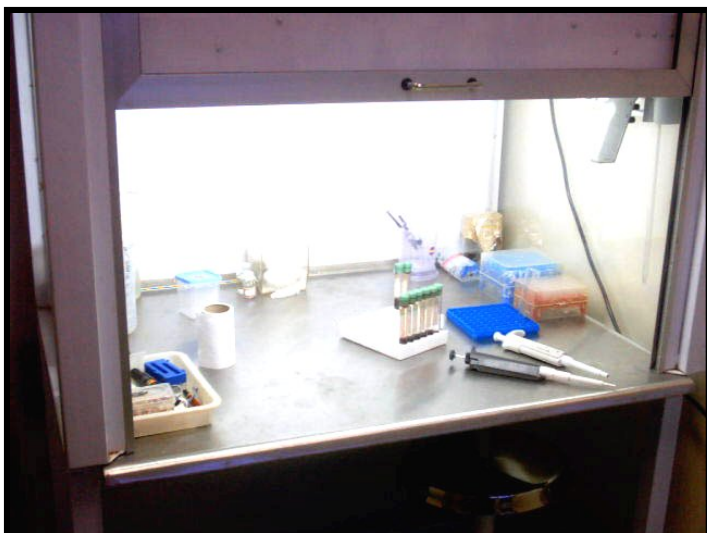
Figure 3: Laminar Air Flow ensures a sterile environment and indirect incandescent lighting conditions
