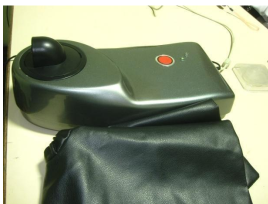
C. EPI Camera pro, which is designed for measuring one finger at a time used in this study. Subjects place their each fingertip, one at a time, on a glass electrode.
