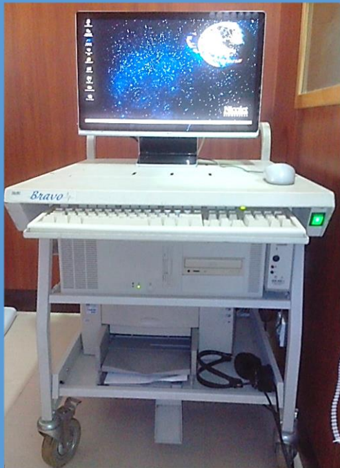
Nicolet Bravo System (Nicolet Biomedicals, U.S.A.) a 4-channel EP acquisition and analysis system with a closed circuit TV on the
